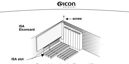
Figure 2. Inserting the Eiconcard C2x.
